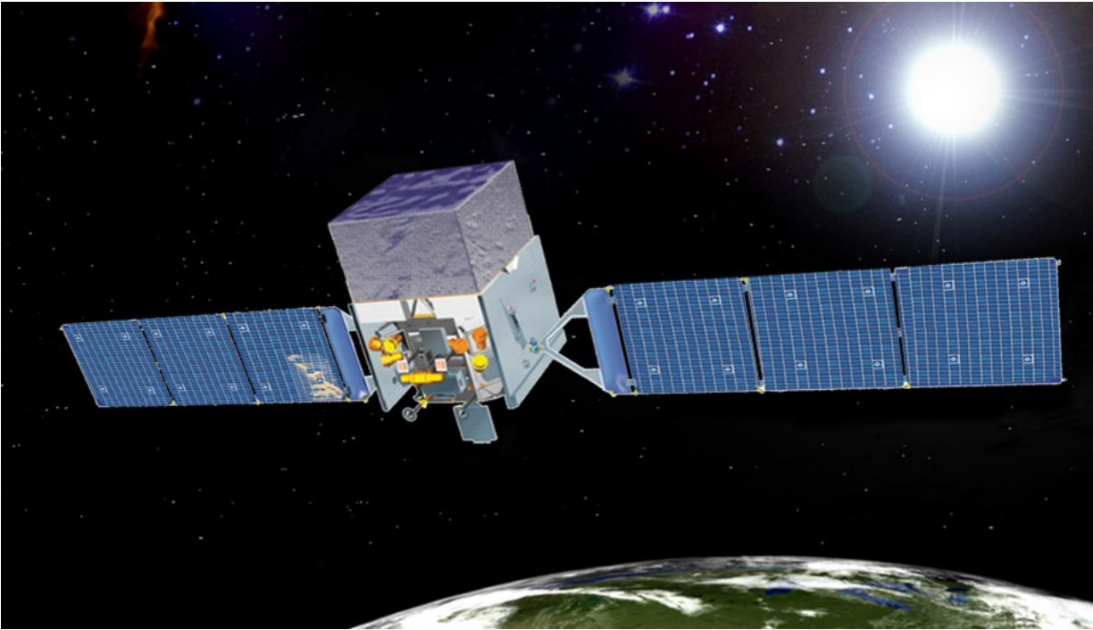
Figure 1.11: An illustration of Fermi in orbit. The cube on the top of the telescope is Fermi-LAT . The GBM is composed of the yellow instruments at the bottom. Source: NASA (original from: fermi.gsfc.nasa.gov ); adapted for this thesis.
