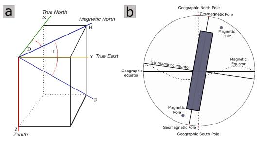
Figure 3. a) Components of Earth's Magnetic Field; b) Comparison between Geographic, Geomagnetic and Magnetic Poles. (modified from Mcelhinny, 1973).
