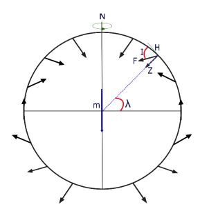
Figure 2. Direction of the Earth's field at the surface following a GAD assumption. The magnetic dipole m is placed in the center of the Earth, aligned with the axis of rotation;  $\lambda$  is the geographic latitude; r is the radius; I is Inclination; and N is the geographic north. Taken and modified from Butler (1992) and references therein.
