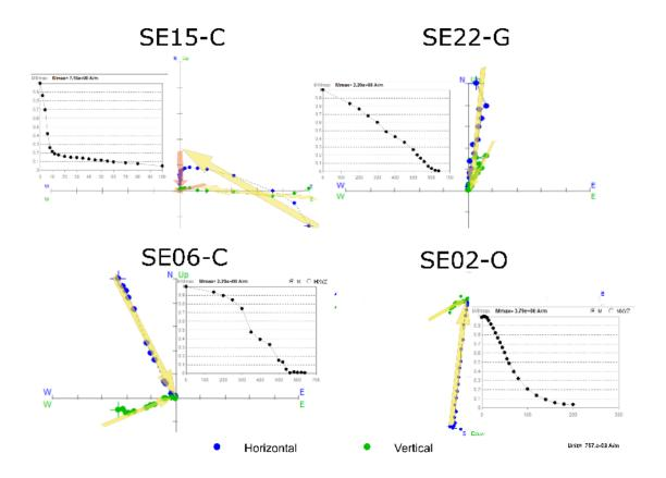
Figure 17. Examples of thermal and alternating field demagnetization diagrams. Zijderveld projections and module plot obtained from SE15, SE22, SE6 and SE2 respectively.
