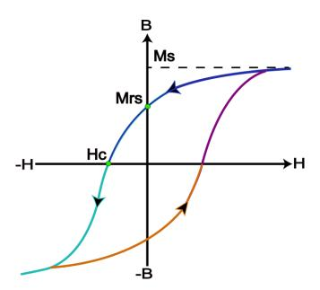
Figure 5. Hysteresis loops. Where H: applied magnetic field; B: induced magnetization; Ms: saturation magnetization; Mrs: remanent saturation magnetization; Hc: coercivity; Hcr: coercivity of remanence.
