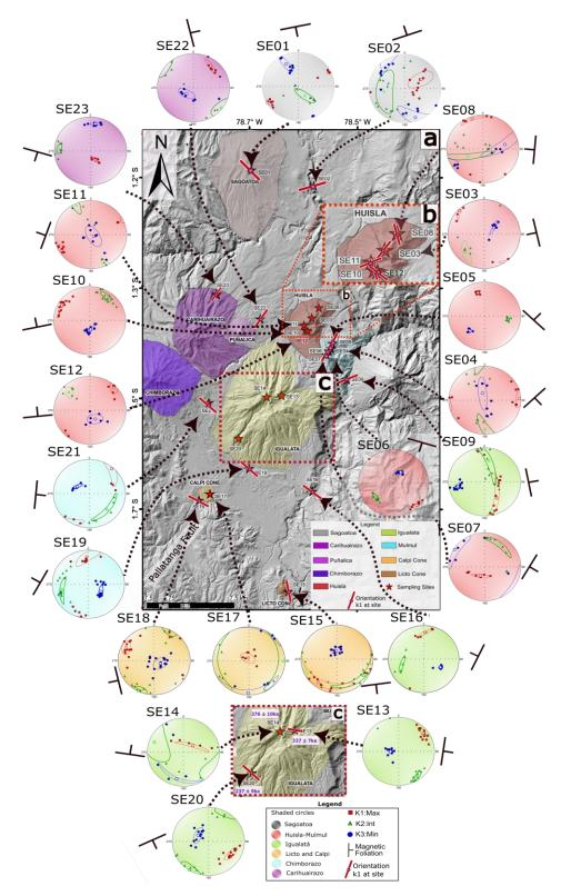
Figure 16. a) Overall AMS directions on a map. The principal susceptibility directions (k1:kmax) are added onto the southern end of the Ecuadorian arc map. The distribution of the magnetic foliations (K<sub>3</sub>) is shown. Where a red square is the k1, a green triangle is k2, and the blue circle is k3; b) red pointed square represents a zoom of the Huisla volcano; and c) red pointed square represents a zoom of the Igualatá volcano.
